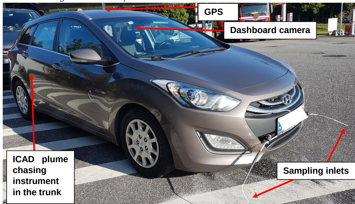
Figure 2: Plume chasing installation on the Danish authority car (outside view). Two sampling inlets are combined to one sampling hose to the ICAD plume chasing instrument in the trunk.
