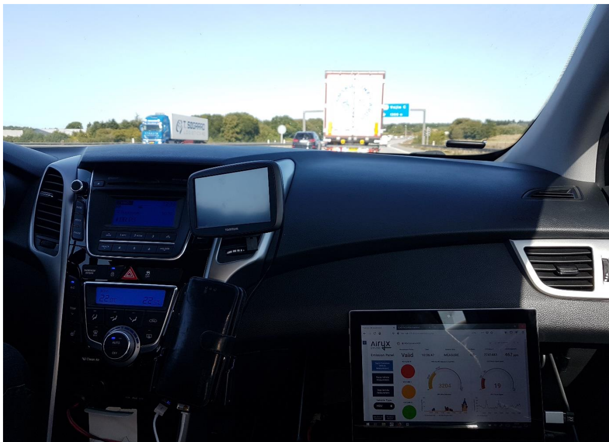
Figure 4: Display installation in the cockpit. A tablet is used as display of the real time data connected via WiFi to the ICAD instrument. It allows operation and visualisation.
